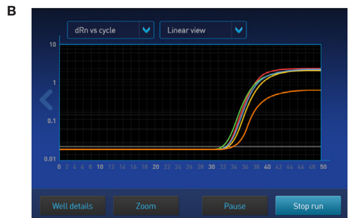
Figure 1. Graphical interface allows (A) easy editing of thermal cycling conditions and viewing of plate layout, as well as (B) viewing of amplification plots and drilling down to a subset of sample wells.
