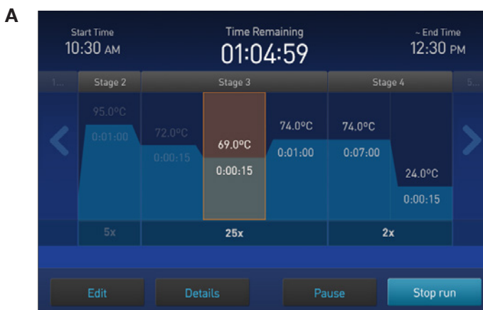
Figure 1. Graphical interface allows (A) easy editing of thermal cycling conditions and viewing of plate layout, as well as (B) viewing of amplification plots and drilling down to a subset of sample wells.
